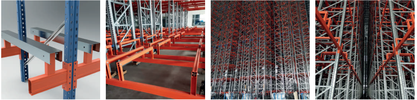
1) Pallet ASRS - Beams with Top Hat for Single or Double storage capacity.
